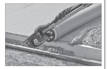
If necessary, handle may be moved to an offset position. Loosen knob (A), remove pins (B) and (C), move handle and handlebar assembly to offset position. Install pin (B) and tighten knob (A). Lower pin (C) will not be used when handle is in the offset position.
